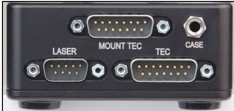
205 TEC Butterfly LaserMount Connectors
