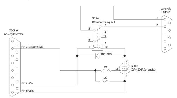
There are many possible choices for the N-channel FET, but it must have the following capabilities: Vds of 5V or greater; current handling of at least 100mA; and a logic-level FET, as the gate voltage will only be 3.3V.
