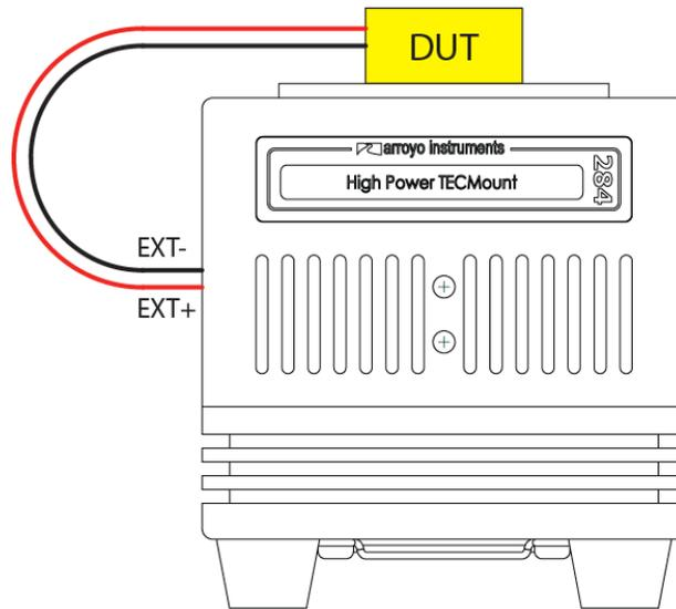
**Wiring of 2-wire sensors**
