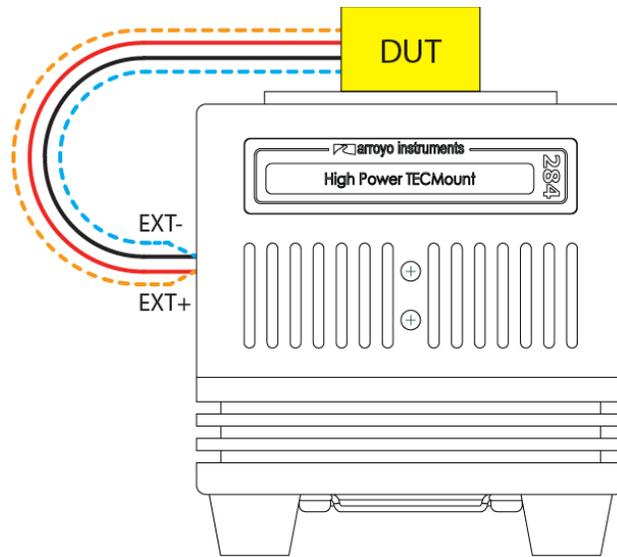
**Wiring of 4-wire sensors**
