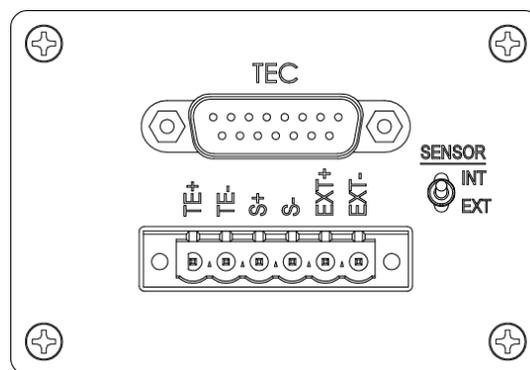
**Example inputs and SENSOR Switch from 284 TECMount**
