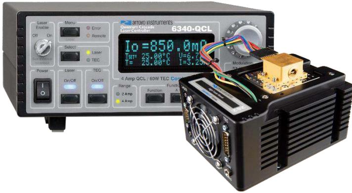
Operation of QCL lasers is very dependent both a stable, low-noise current source for the laser plus the ability to control the temperature of the laser chip across a wide range, as temperature, combined with current, determines the operating frequency of the QCL laser. Thermal control can often be one of the more challenging aspects of the system due to the wide temperature range required of the QCL laser.
