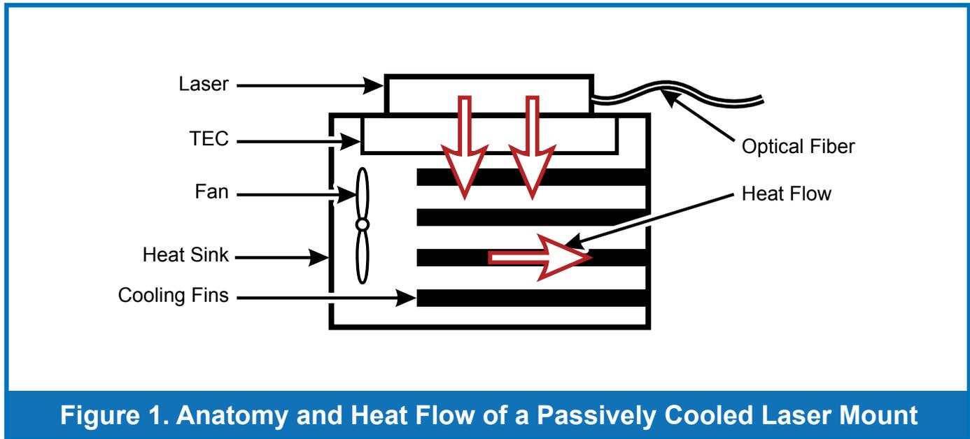
A fan will improve the thermal performance of a passively-cooled laser mount. Typically, the manufacturer will provide ratings for the laser mount with and without an auxiliary fan. Even with a fan, the performance and power range of a passive heat sink are limited to low- and medium-power applications, or applications where higher operating temperatures are acceptable.
