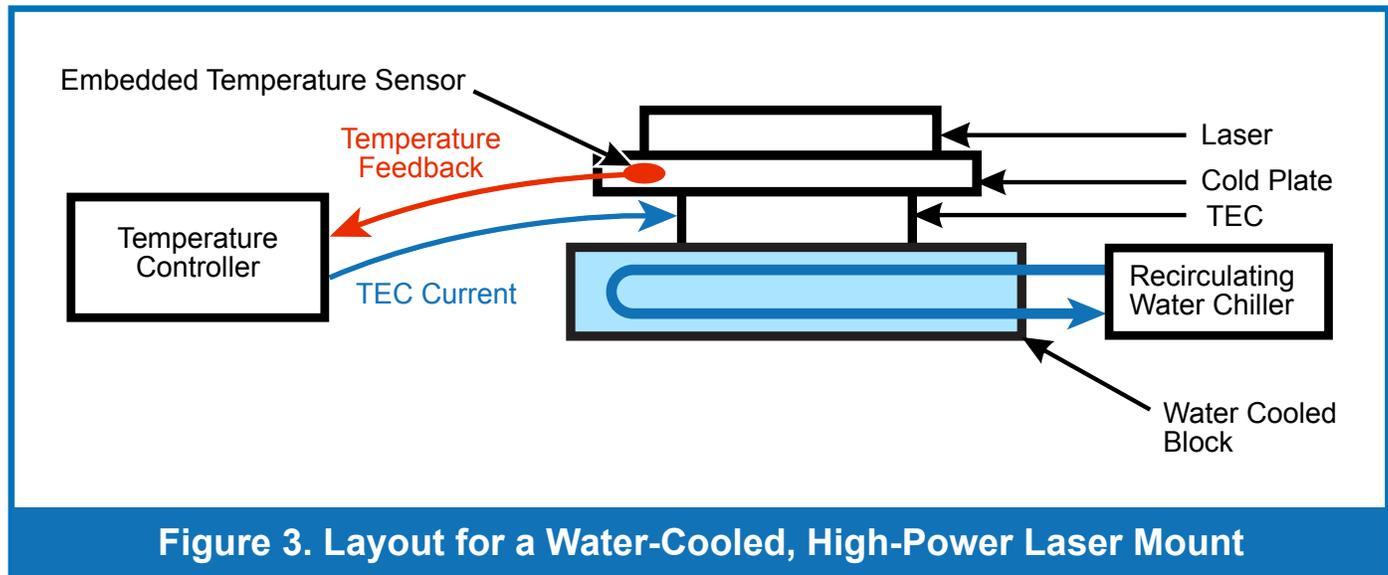
Figure 3. Layout for a Water-Cooled, High-Power Laser Mount
