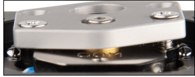
BAD: Diode improperly clamped, clip is uneven with cold plate
