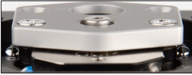
GOOD: Diode properly clamped, clip is even with cold plate
